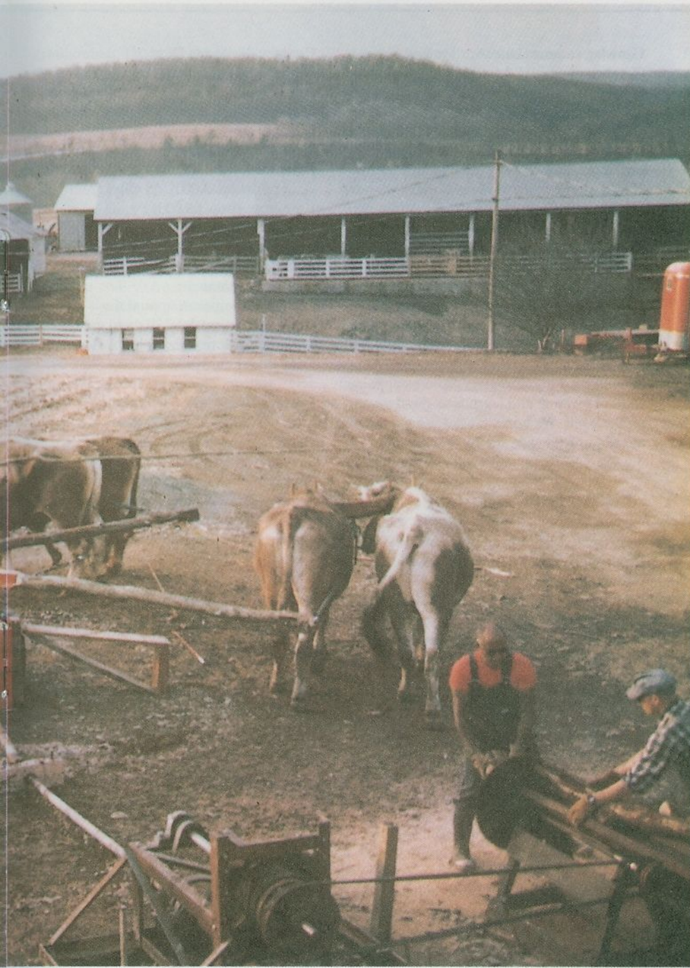
An ox-driven sawmill at Gītā Nāgari demonstrates one of many uses for oxen. As the oxen walk in a circle, a mechanism of pulleys, shafts, and gears delivers the power generated by the oxen to the saw at the lower right of the picture.
